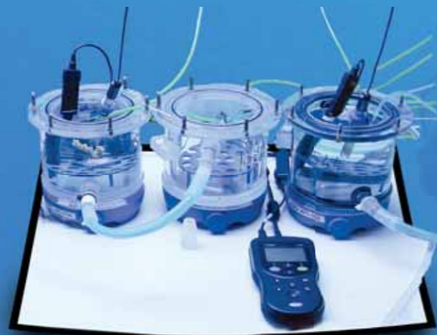
Laboratory setup for coral calcification measurements. Oxygen, pH and temperature probes allow a tight control over environmental conditions. © T. Wijgerde - Wageningen UR).
