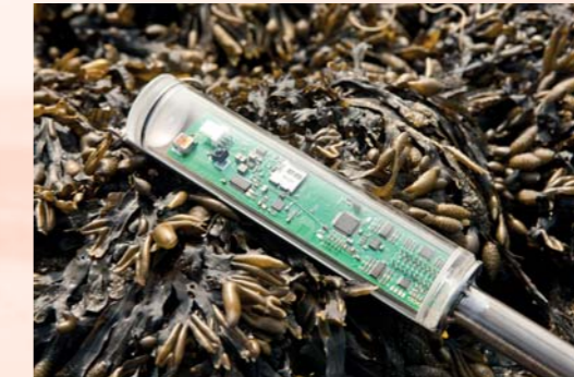
The upper part of the sediment meter.
