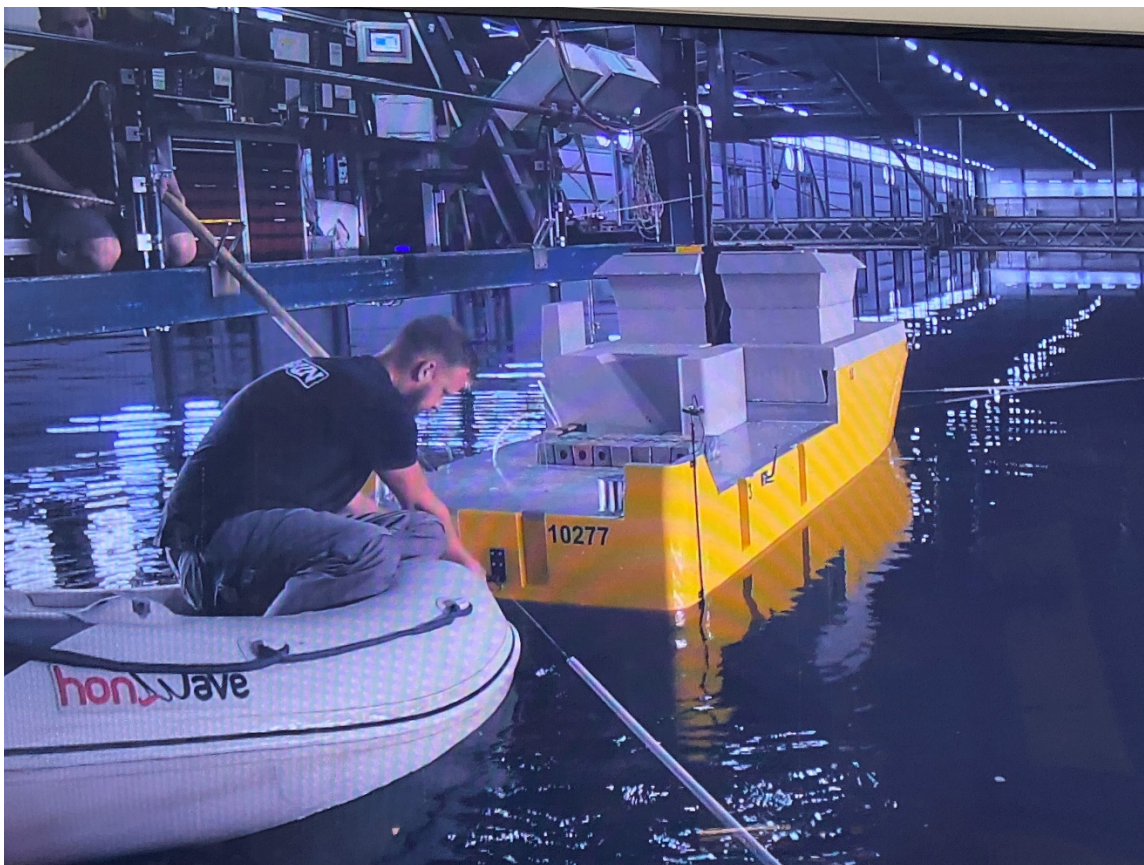
A MARIN technician uses a rubber boat to disconnect the model from the 'train' to allow it to sail under its own power. A second technician on the 'train' holds the model in place with a boat hook.
