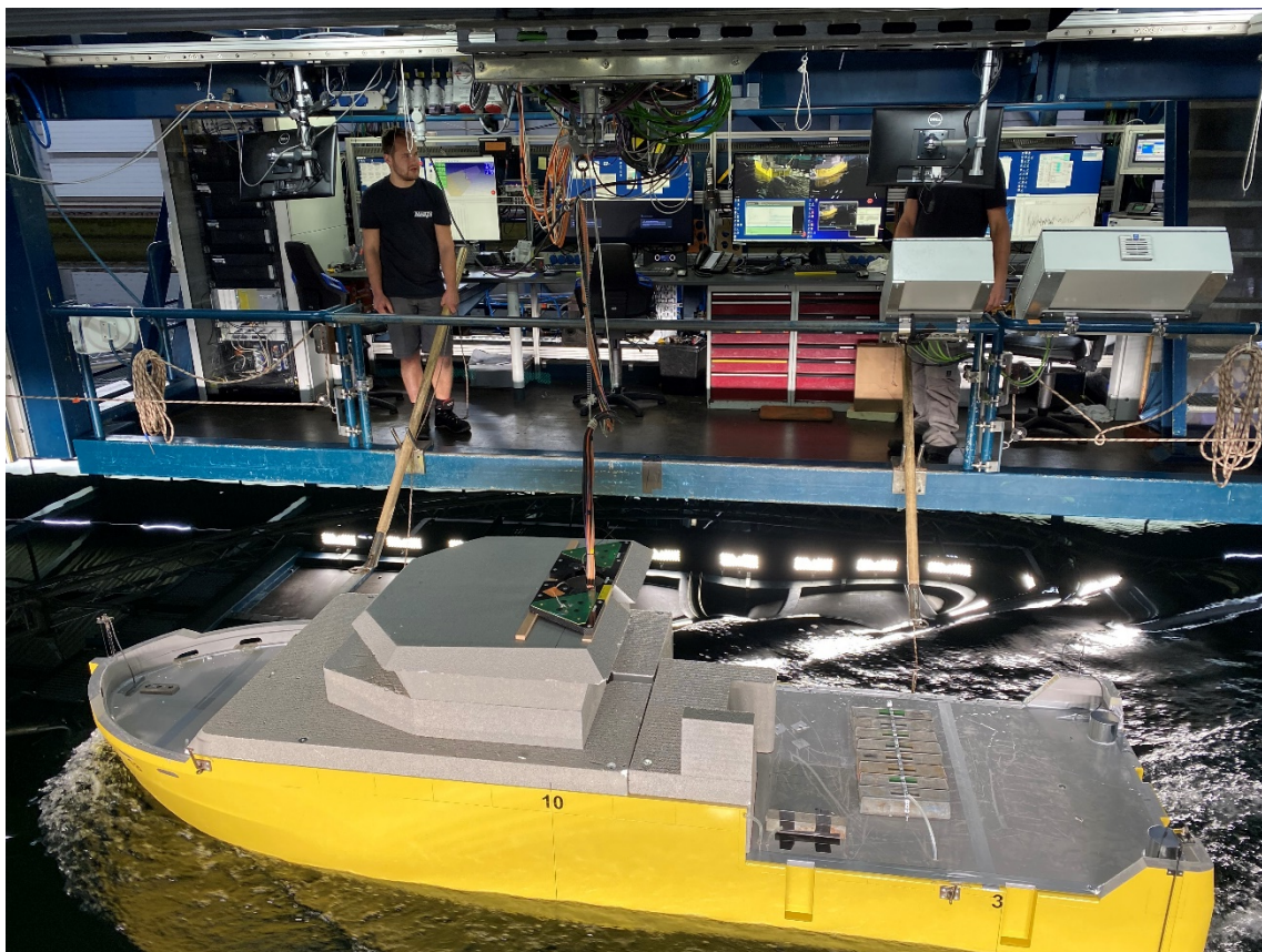
The model is held in place with boat hooks until it reaches the desired speed under its own power.
