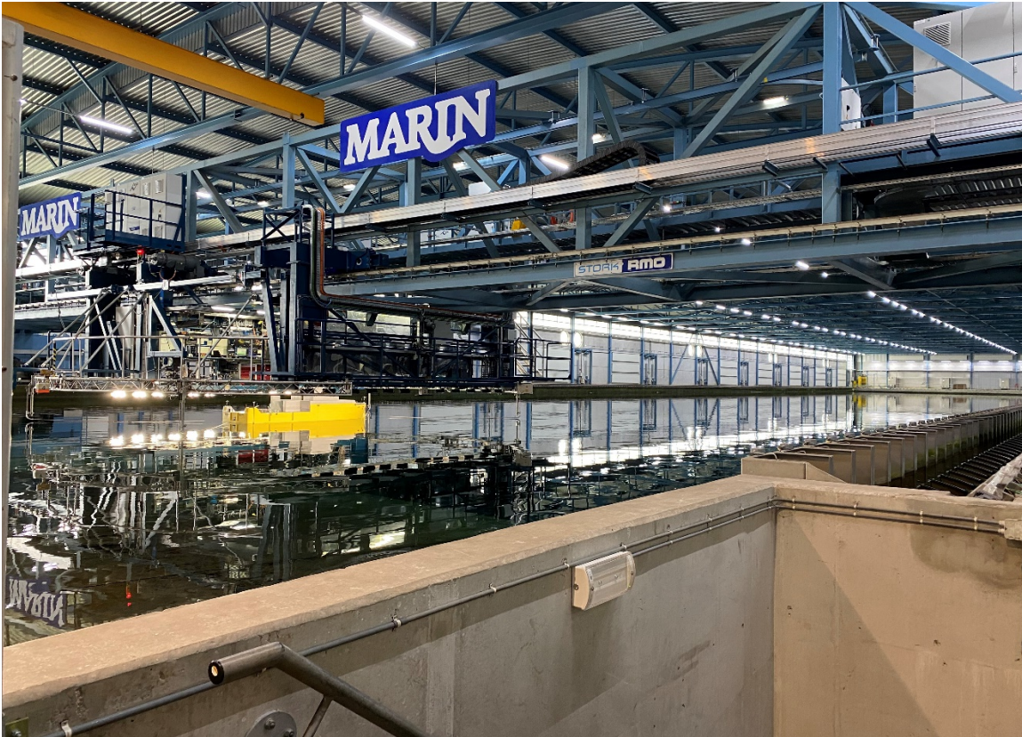
MARIN sea handling test basin. The moveable wall panels that generate waves can be seen at the right. The yellow test model of the RV Wim Wolff can be seen in the middle of the drag tank, below the 'train'; the frame used to operate the measurement instruments and a viewing platform.
