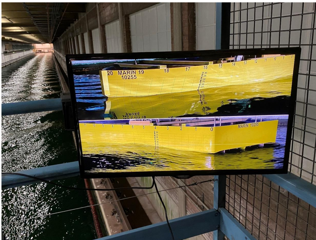
The towing tank at MARIN in Wageningen with on the screen the scale model of RV Wim Wolff .
