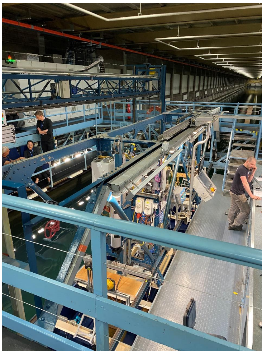
The carriage, the frame over the towing tank with in the middle the scale model of RV Wim Wolff, on the right the operator with the measuring equipment; on the left the grandstand with interested parties.
