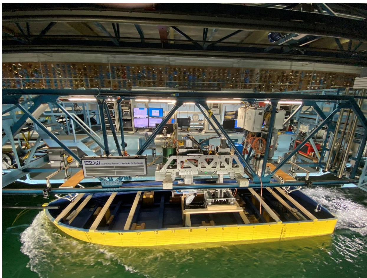
Towing model of RV Wim Wolff during a test run
