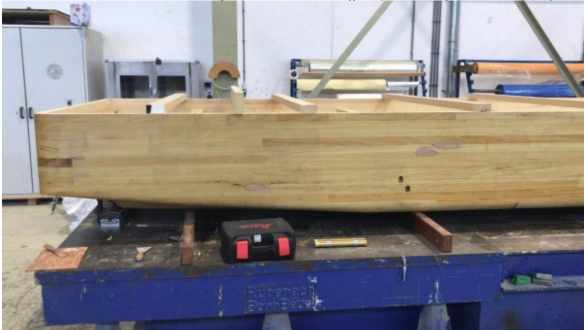
Construction of the hull model for the RV Wim Wilff for the drag tank test at MARIN. ©TBG
