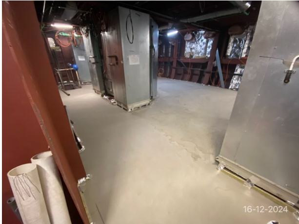
Concrete deck treatment on the F-deck and insulation against the outer hull.
