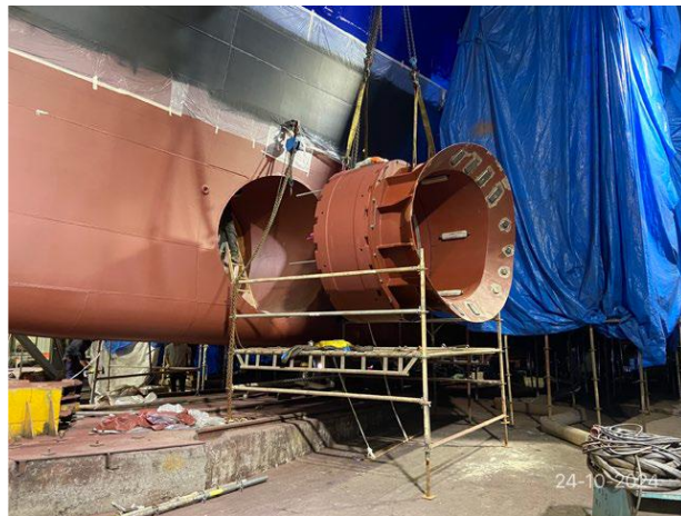
Installation of the bow thruster
