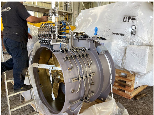
Bow thruster with air injection
