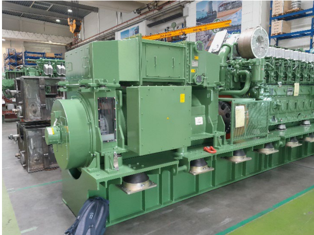
ABC 8-cylinder generator set
