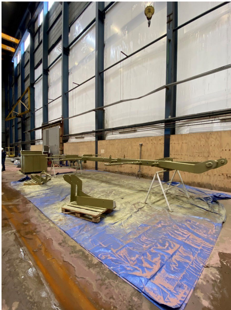
The radar mast primed and ready for further assembly
