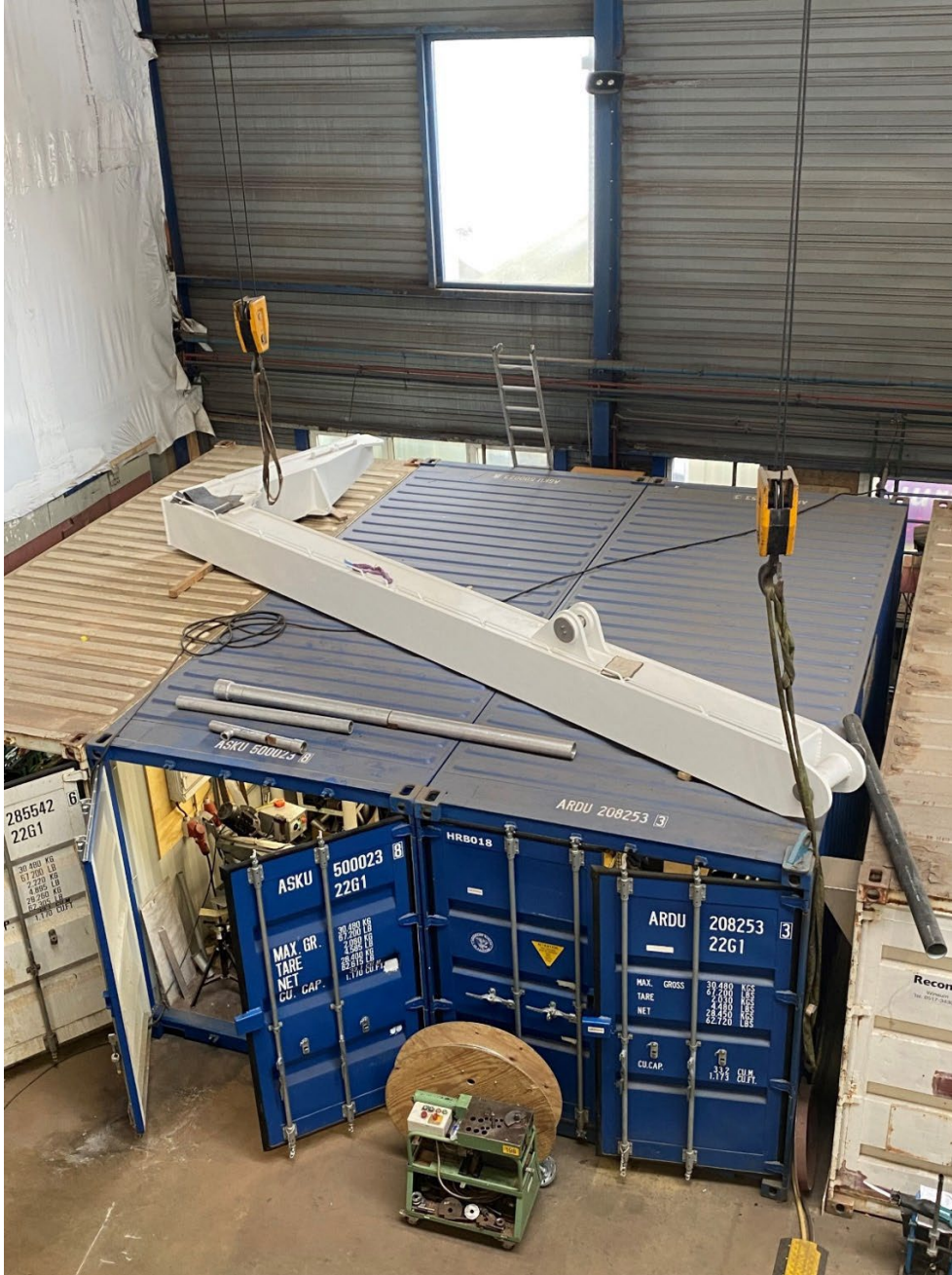
The J-frame, ready to be installed
