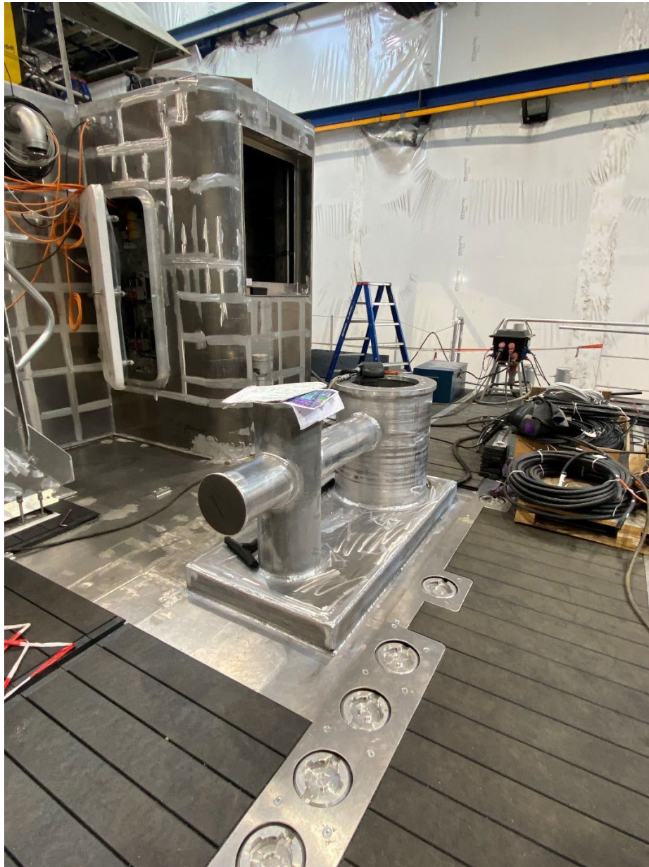
The capstan installed on the aft deck, showing the cylinder for the reel drum.
