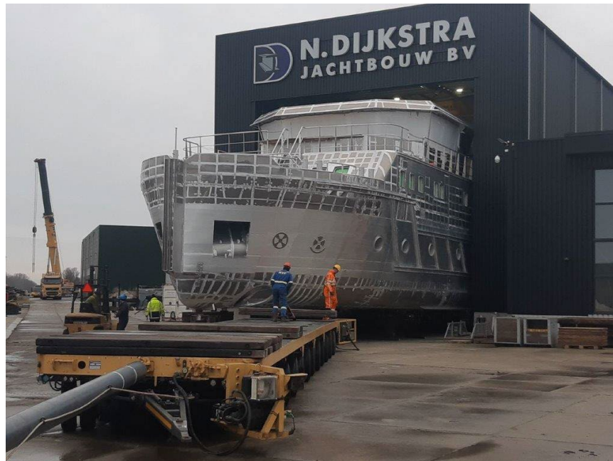
The hull of the RV Wim Wolff, showing preparations for transport. ©FH
