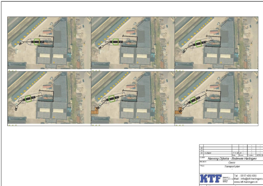
Detailed transport plan for moving the hull from the hall at Dijkstra shipyard, showing the limited range of movement. ©KTF
