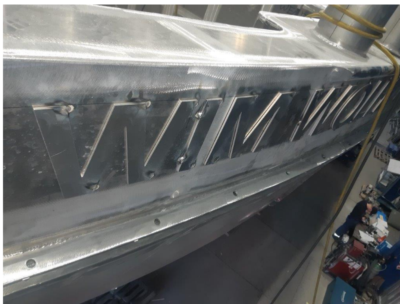
The letters of the vessel's name have been welded to the hull. ©FH
