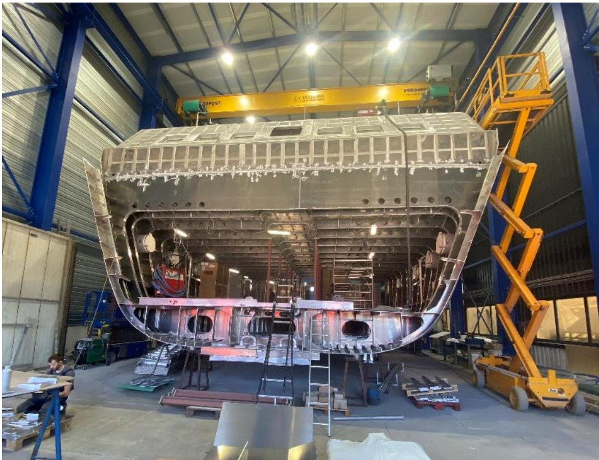
Front view of the RV Wim Wolff, with the pipe tunnel visible behind the ladder.
