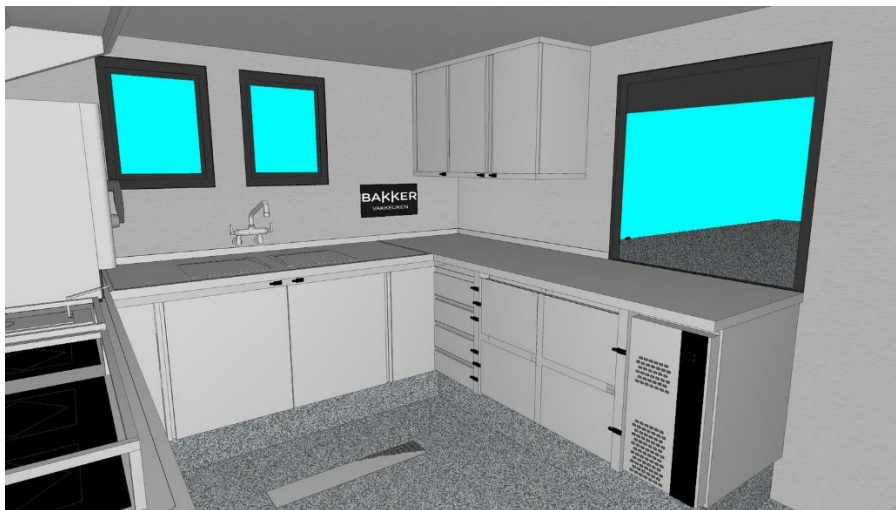
Revised sketch of the galley aboard the RV Wim Wolff. The serving hatch to the messroom is shown to the right.
